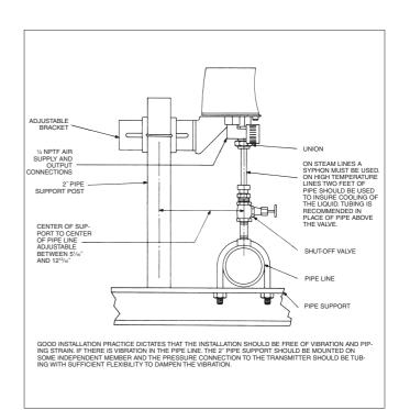
Figure 5. Pipe-Mounted Pressure Transmitter Installation
