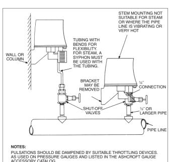
DIAPHRAGM SEALS MAY BE INSTALLED DIRECTLY TO THE TRANSMITTER OR WITH A CAPILLARY LINE. (BOURDON TUBE ELEMENTS ONLY. SUPPLY AND OUTPUT AIR CONNECTIONS ARE ¼ NPT FEMALE. DRAIN OR VENT VALVES SHOULD BE INSTALLED ABOVE THE SHUT OFF VALVE ON HIGH PRESSURE GAS OR DANGEROUS LIQUID INSTALLATIONS.
