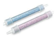
Over time, the desiccant will change from blue to pink as each filter becomes saturated with water. (see picture). When the unit is pink, the ability to filter moisture is likely affected and should be replaced. The expected duration for this replacement would be highly dependent on the environmental conditions.
