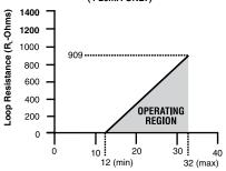
Loop Supply Voltage (Vdc) [LSV]
