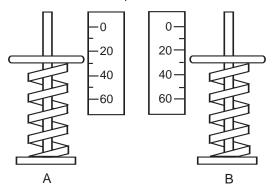
**Series PP-D Dual Switch** – Remove front cover, held in place by two screws. There are two range adjusting wheels. The adjusting wheel on the left (labeled A) controls the left switch, the adjusting wheel on the right (labeled B) controls the right switch. The switches are set independently.
