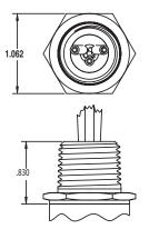
FLYING LEADS ELECTRICAL TERMINATION CONDUIT - 1/2 NPT MALE (C2), (C5)
