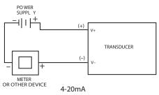
A4 transducer has internal transient protection: for safety, limit line-to-ground voltage to 36 Vdc max.
