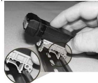
Figure 7. Snapping the Module to the DIN Rail
