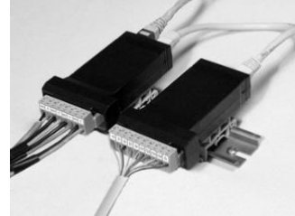
Figure 6. Examples of Modules Mounted to DIN Rail
