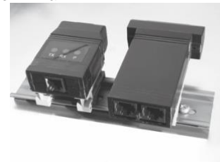
Figure 8. Typical Installation of DIN Rail Mounted Devices
