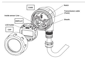
Turn display over to expose terminal strip, make positive and negative connections, insert wire depth is equal to recommended strip length (0.25").
