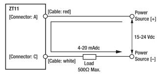
When connecting equipment that can generate surge from the same power supply, it is recommended that a voltage-dependent resistor (varistor) be connected to the pressure transmitter for protection. In addition, take the following precautions when wiring:
