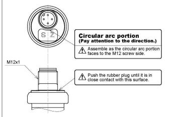
The "Z" on the rubber plug indicates the position of the potentiometer for zero adjustment, and the "S" indicates the position of the potentiometer for span adjustment.
