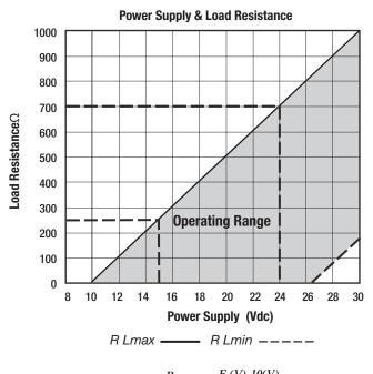
Maximum load resistance $R_{Lmax}$  $\frac{E(V)-10(V)}{0.02(A)}(\Omega)$ Vinimum load resistance $R_{Lmin}$  $\frac{E(V)-26.4(V)}{0.02(A)}, R_{Lmin \ge o(\Omega)}$
