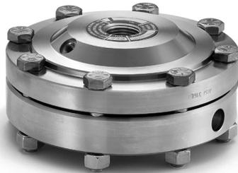
A change in pressure at the process connection causes a displacement of the filling fluid due to deflection of the diaphragm, transferring the change in pressure to the sensing element of the pressure instrument.
