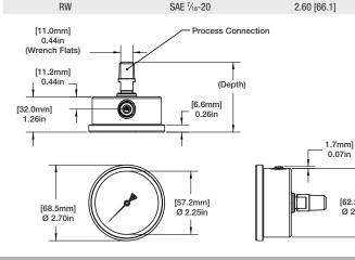
63 mm center back connect - connection mounted U-clamp **Connection Code Process Connection** Depth 01 1% NPT 2.36 [60.0] 02 1/4 NPT 2.50 [63.4] 13 G¼ B 2.49 [63.3] 41 M14x1.5 2.53 [64.3] JIC #4 EJ 2.44 [62.0] JP 1/4 Tube 2.60 [66.1] JR 3% Tube 2.73 [69.4] JS 1/2 Tube 2.86 [72.7] KA 1/4 BSPT 2.42 [61.4] RW SAE 7/16-20 2.60 [66.1]
