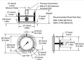
63 mm center back connect - front flange, case mounted U-clamp **Connection Code Process Connection** Depth 01 1/8 NPT 2.36 [60.0] 02 1/4 NPT 2.50 [63.4] 13 G¼ B 2.49 [63.3] 41 M14x1.5 2.53 [64.3] EJ JIC #4 2.44 [62.0] JP 1/4 Tube 2.60 [66.1] JR 3% Tube 2.73 [69.4] JS 1/2 Tube 2.86 [72.7] 1/4 BSPT KA 2.42 [61.4] RW SAE 7/16-20 2.60 [66.1] [49.2mm] Process Connection [11.0mm]
