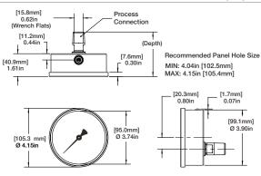
100 mm lower back connect - case mounted U-clamp **Connection Code Process Connection** Depth 1/4 NPT 02 3.13 [79.5] 04 1/2 NPT 3.13 [79.5] 09 1/4 HP Female 3.13 [79.5] 13 G1⁄4 B 3.13 [79.5] 15 G1⁄2 B 3.26 [82.8] 16 M20x1.5 3.26 [82.8] JP 1/4 Tube 3.13 [79.5] JR 3% BSPT 3.25 [82.6] JS 1/2 Tube 3.38 [85.9] KA 1/4 BSPT or R 1/4 3.13 [79.5] KD 1/2 BSPT or R 1/2 3.14 [79.8]
