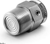
A change in pressure at the process connection causes a displacement of the filling fluid due to deflection of the diaphragm, transferring the change in pressure to the sensing element of the pressure instrument.
