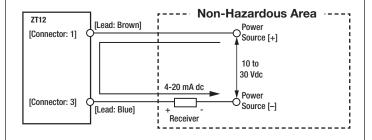
When connecting equipment that can generate surge from the same power supply, it is recommended that a voltage-dependent resistor (varistor) be connected to the pressure transmitter for protection. In addition, take the following precautions when wiring:
