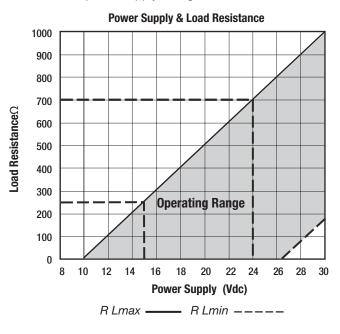
Maximum load resistance  $\frac{R_{Lmax}}{0.02(A)} = \frac{E(V) - 10(V)}{0.02(A)} (\Omega)$
