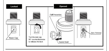
The rubber plug is equipped with a simple tethering function, however if it is pulled too strongly, it may be damaged. Please be careful not to use more force than necessary [<17 in. lb.].</li>
